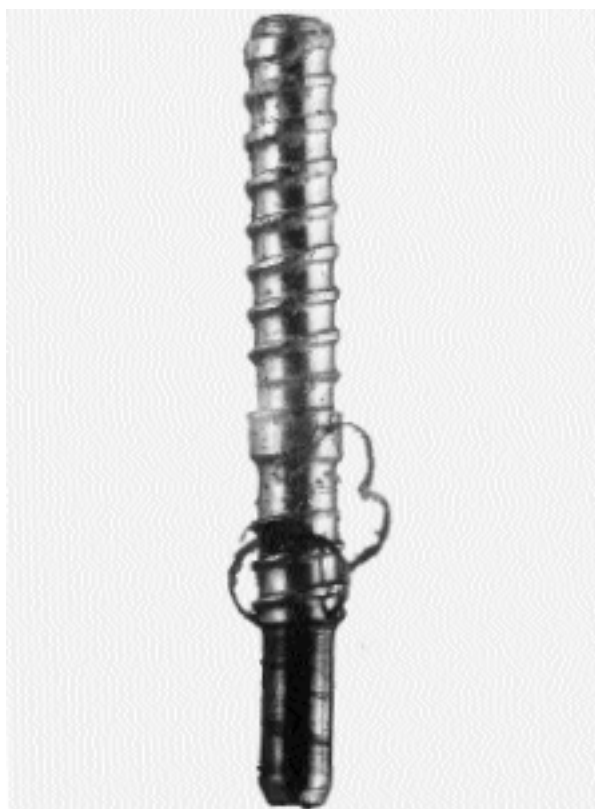
Fig. 1.—Stripping of TMS Link Plus Minim pin when placement attempted in pinhole prepared with 0.48 mm drill bit.
