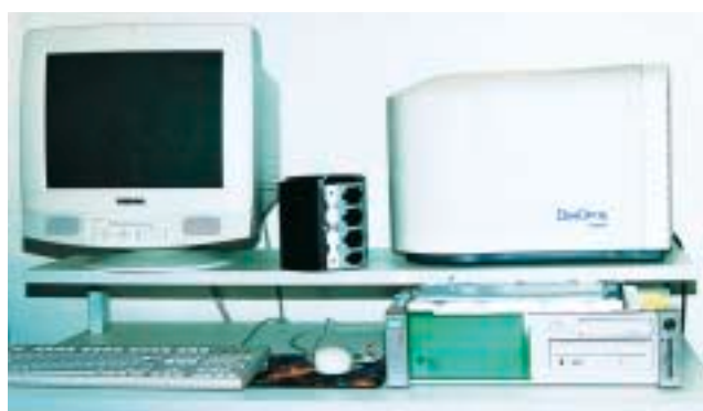
Fig 5. DenOptix imaging plate system hardware. Periapical and panoramic films are placed on a cylindrical insert that rotates within the laser beam scanner/processor.
