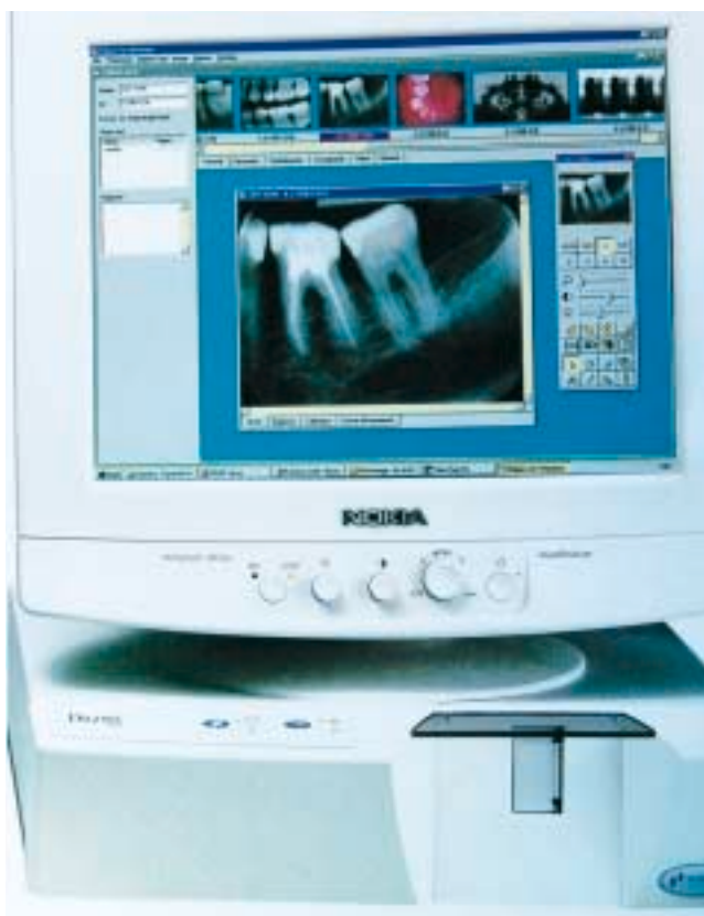
Fig 3. Digora fmx hardware. Processor add-ons cope with full mouth survey or high volume film taking.
